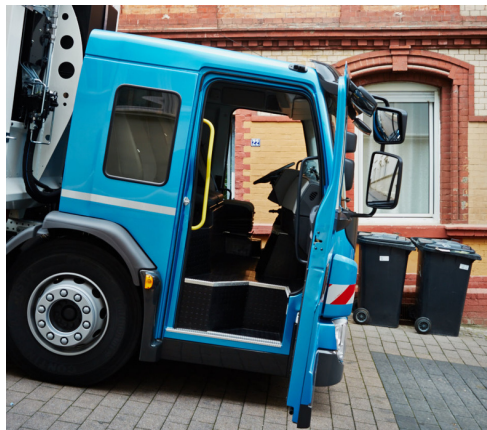
Easy and safe entry and exit with large anti-slip footstep and flat floor. Picture showing STWPOS-L.
