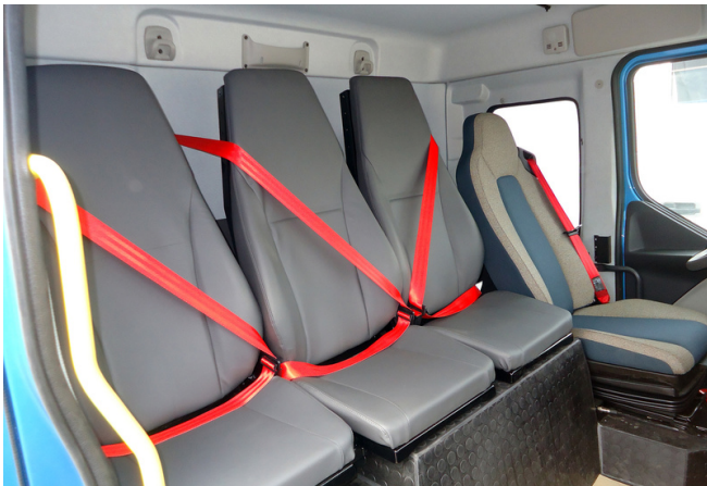
1+3 version as option. Comfortable seats for three passengers (S90095), including coat hanger behind driver's seat as well as red seat belts (S90909). Picture showing STWPOS-L.
